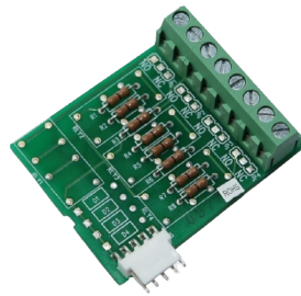
OC Extension Module
